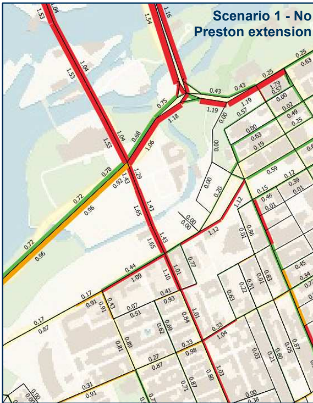
Figure 23: PM Peak Hour EMME Model v/c Ratio
