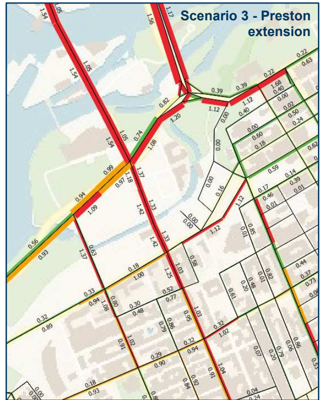
Figure 23: PM Peak Hour EMME Model v/c Ratio
