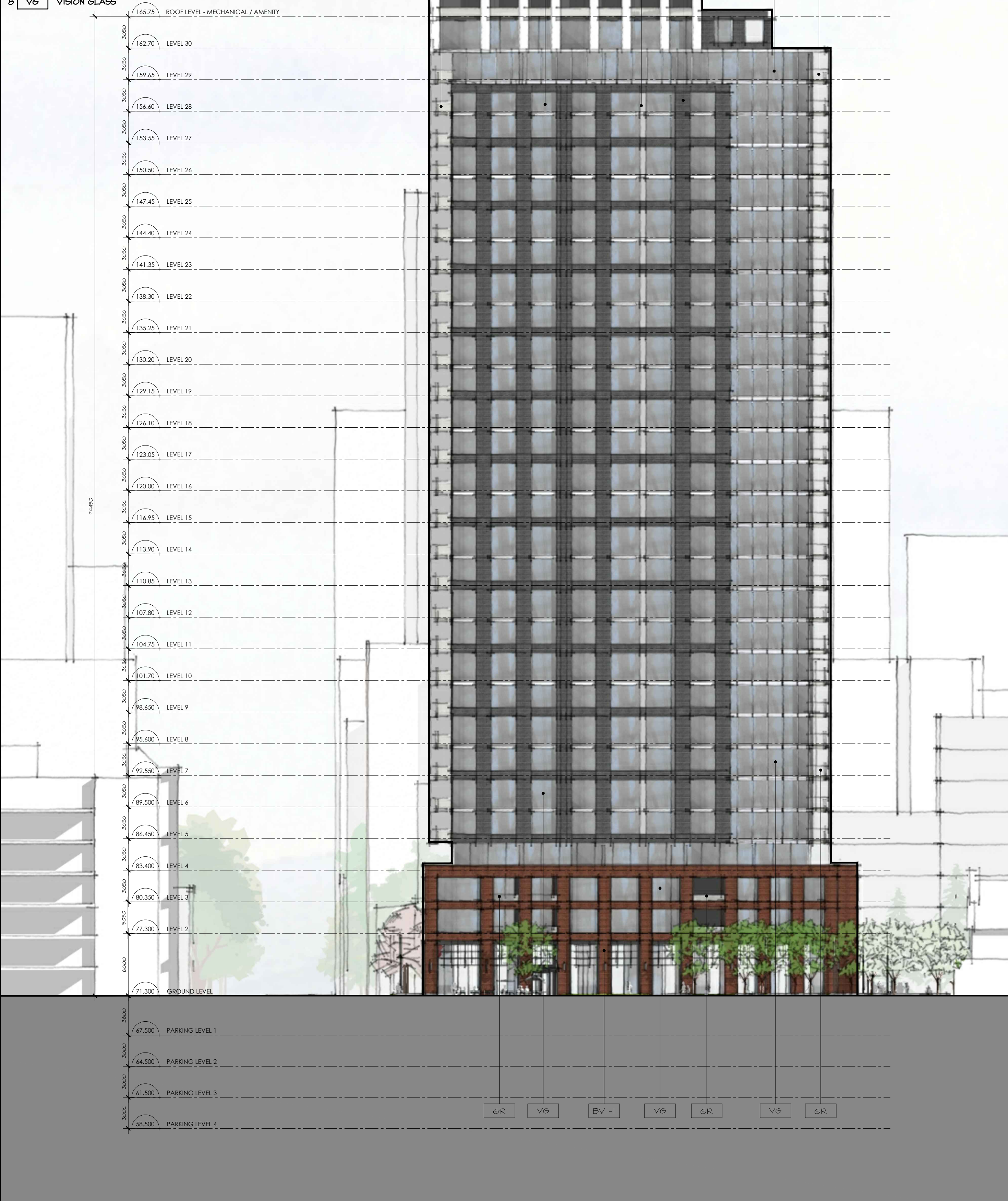
A3.02 NORTH TOWER – SOUTH ELEVATION A3.02 1:150
