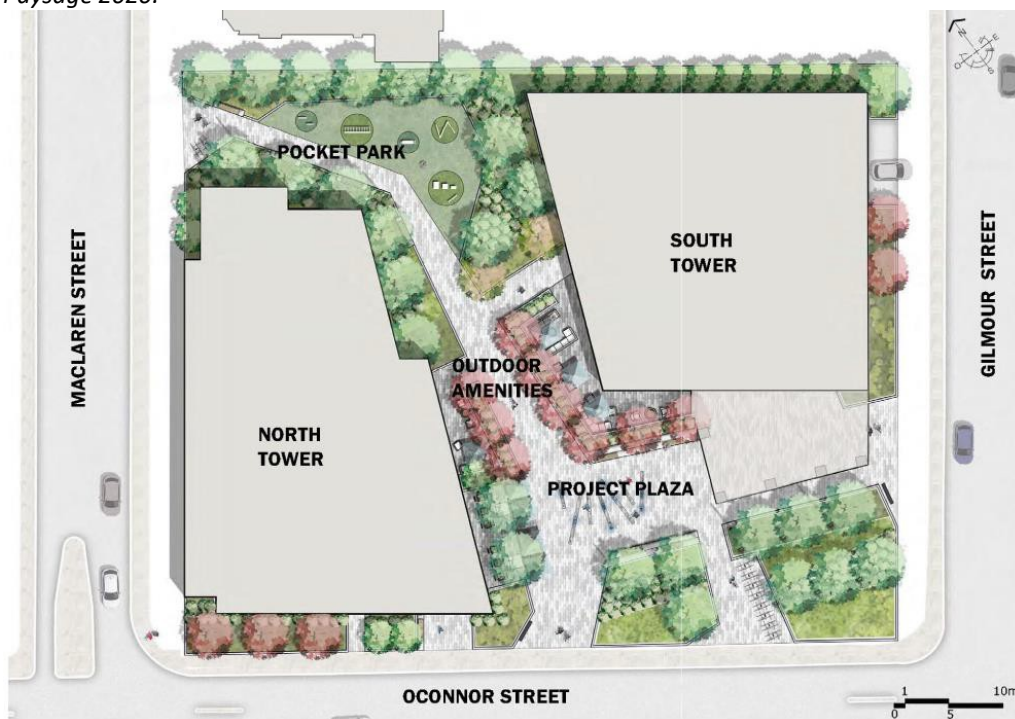
Figure 19: Site plan of the proposed development illustrating the proposed landscape treatment and circulation pattern within the site. Source: Projet Paysage 2020 .
