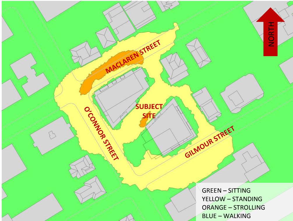
FIGURE 3A: SPRING – WIND CONDITIONS AT GRADE LEVEL
