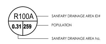
SANITARY DRAINAGE AREA ID# INFILTRATION RATES
