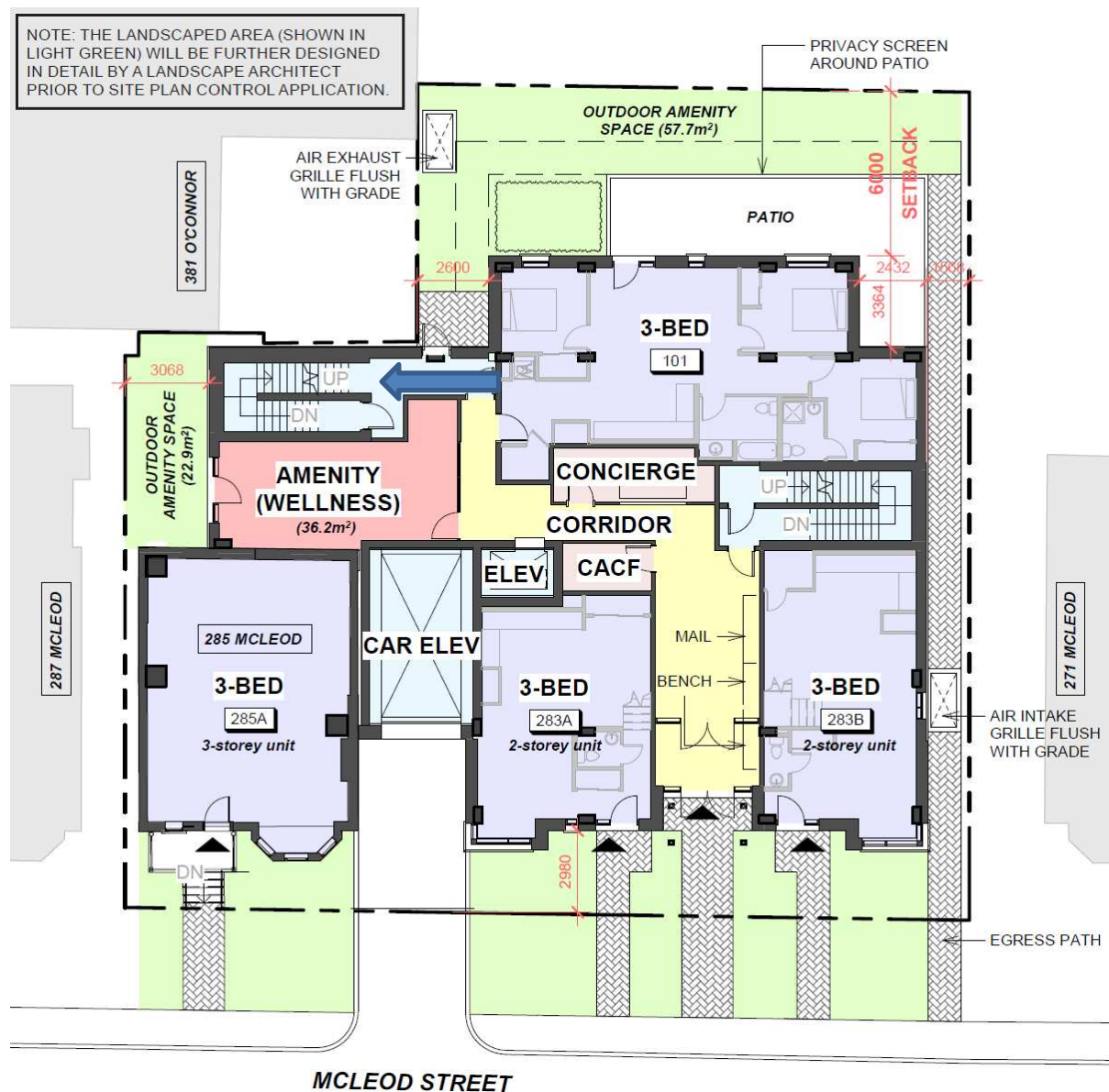
Figure 25: Plan view of the development site illustrating the building setbacks. Soft landscape is limited to the front of the building, and the sidewalk street trees are not shown. The mid-rise is setback over the façade of the 285 to allow it to continue to be interpreted as part of the streetscape.
