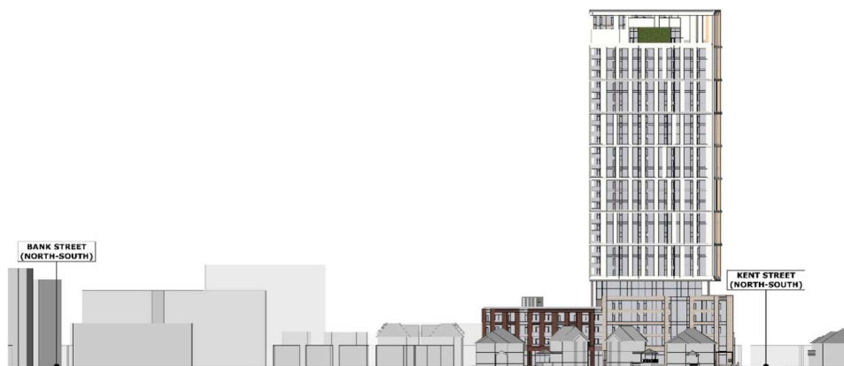
Figure 13: Proposed transition along MacLaren Street (Looking South). The new podium (shown in red) is set at four storeys and clad in traditional red brick acknowledging neighbouring homes. Source: Hobin Architecture 2023.
