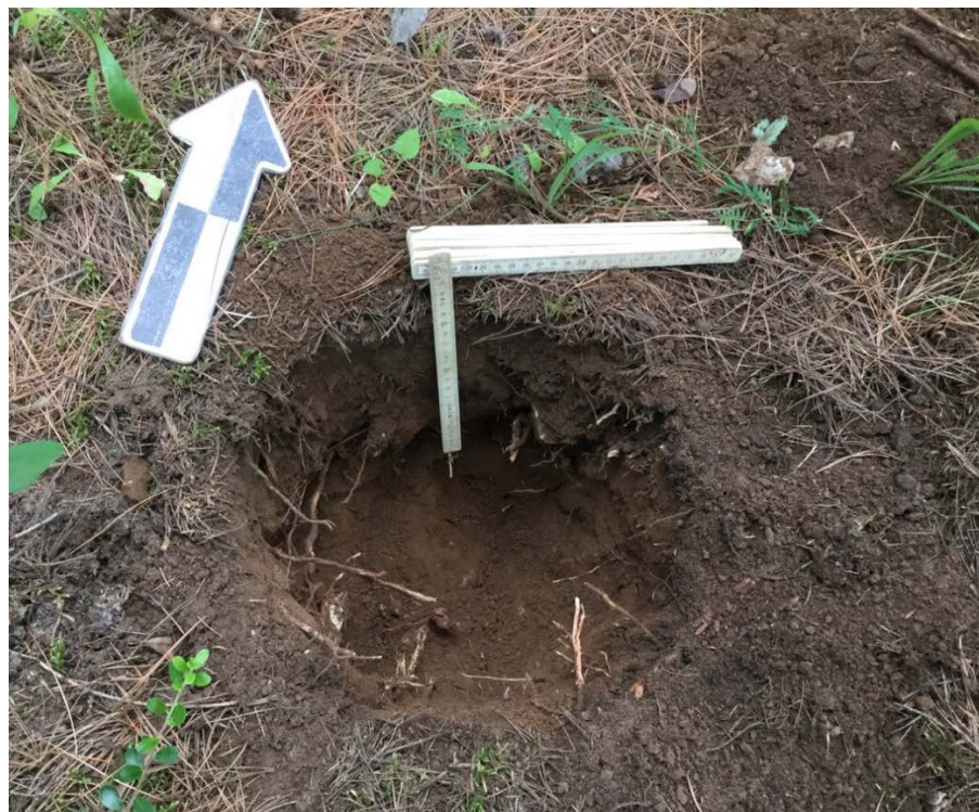
Image 12: Soils in Operation 3 consisted of medium brown sandy loam topsoil above light orange-brown subsoil.
