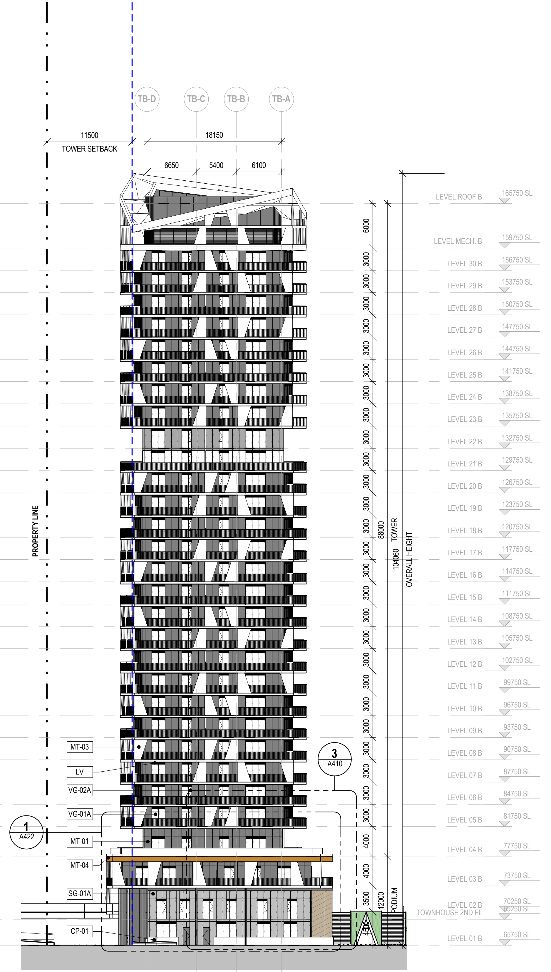
1 TOWER B NORTH ELEVATION 1:300
