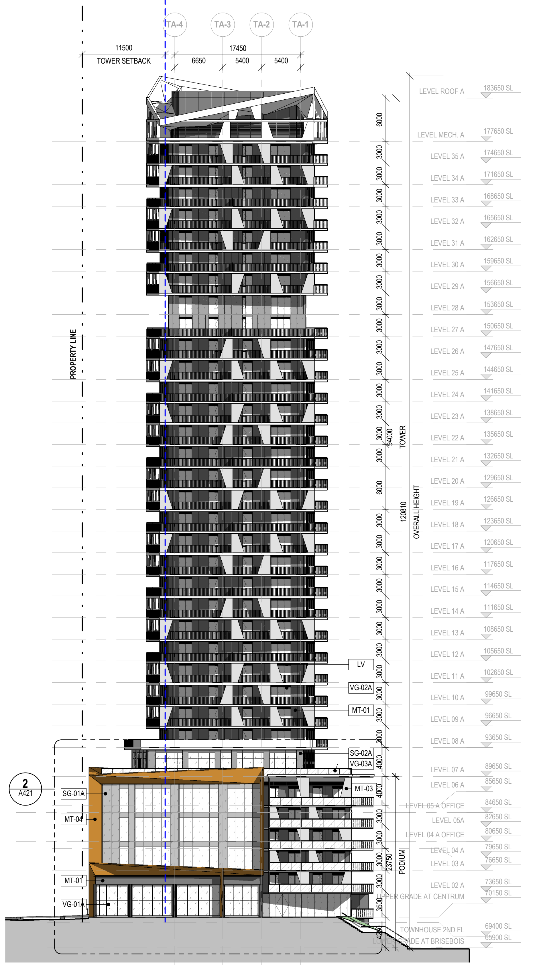
2 TOWER A EAST ELEVATION 1:300
