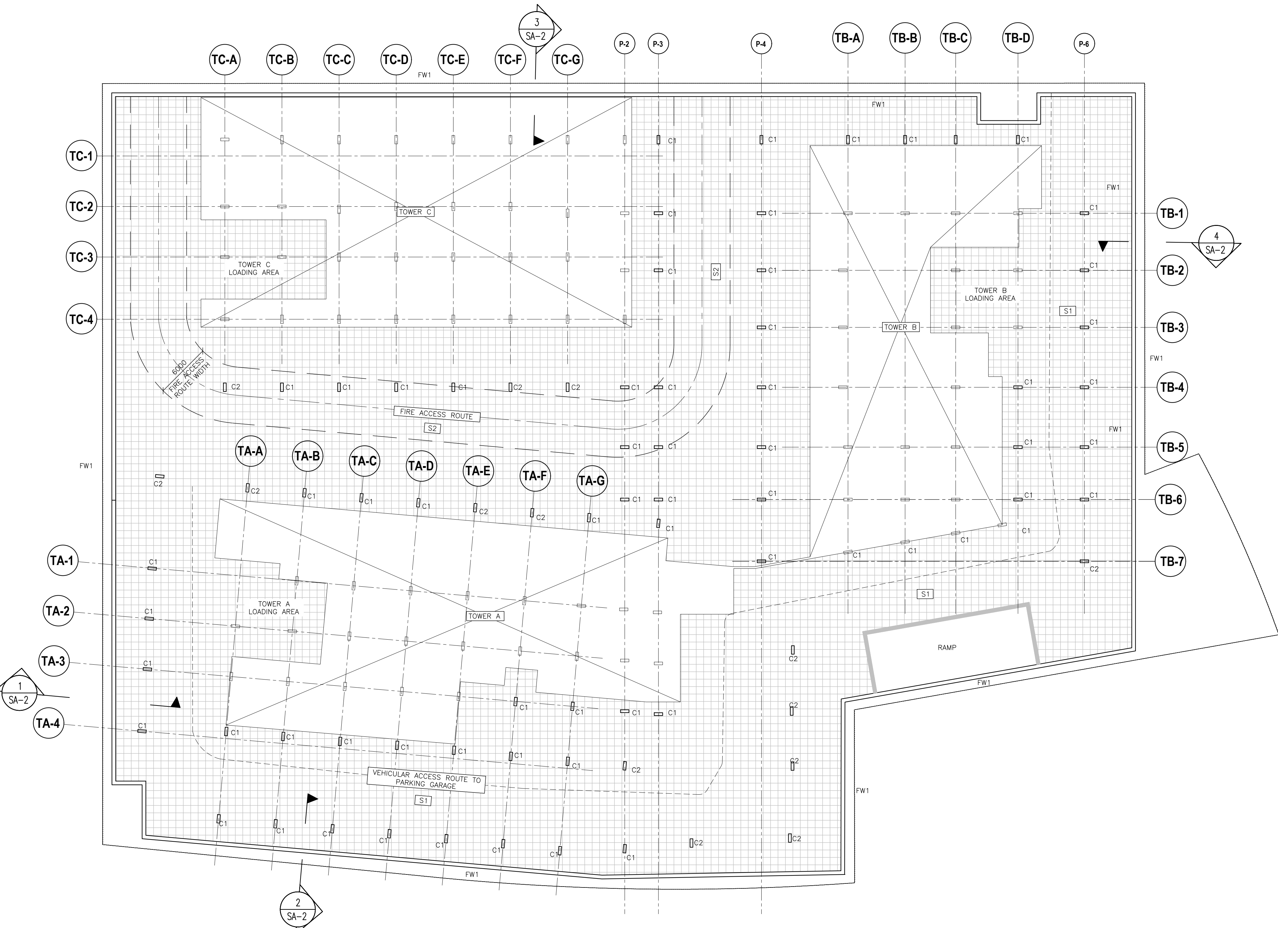
1 SA-1 1:250 1 PARKING GARAGE P1 ROOF PLAN
