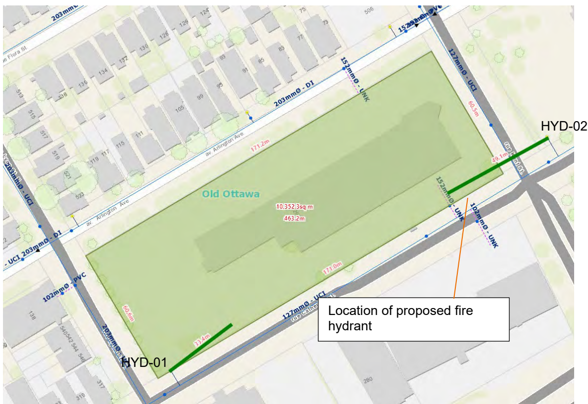
Figure 3-1: Fire Hydrant Coverage Sketch
