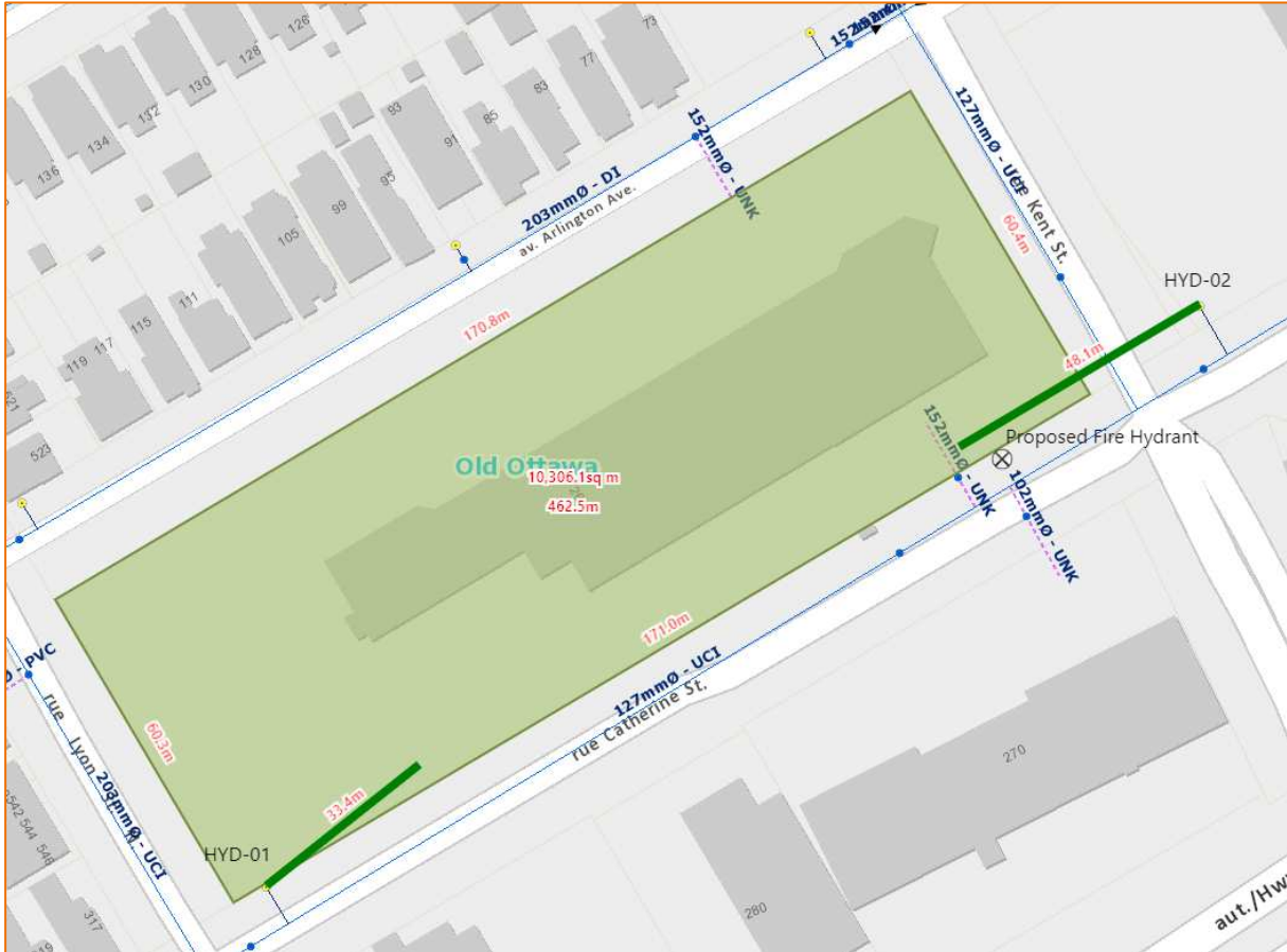
Figure 3.1: Fire Hydrant Coverage Sketch
