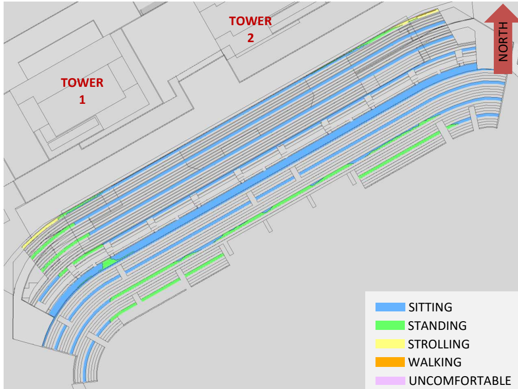
FIGURE 30A: WINTER – WIND COMFORT, SELECT NEW NSS ROWS WITH NSS ROOF
