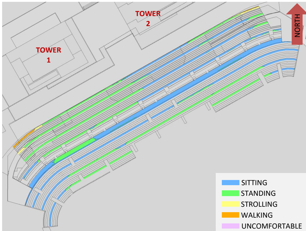
FIGURE 30B: WINTER – WIND COMFORT, SELECT NEW NSS ROWS WITHOUT NSS ROOF
