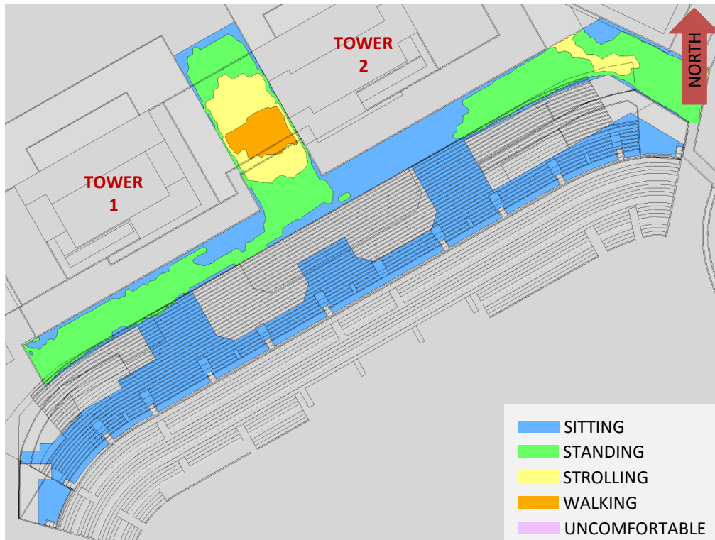
FIGURE 11B: SPRING – WIND COMFORT, PROMENADE LEVEL WITHOUT NSS ROOF
