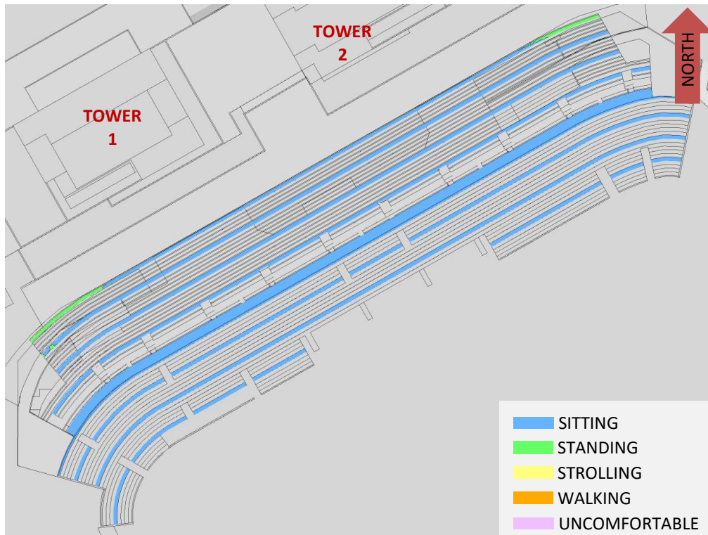
FIGURE 28B: SUMMER – WIND COMFORT, SELECT NEW NSS ROWS WITHOUT NSS ROOF
