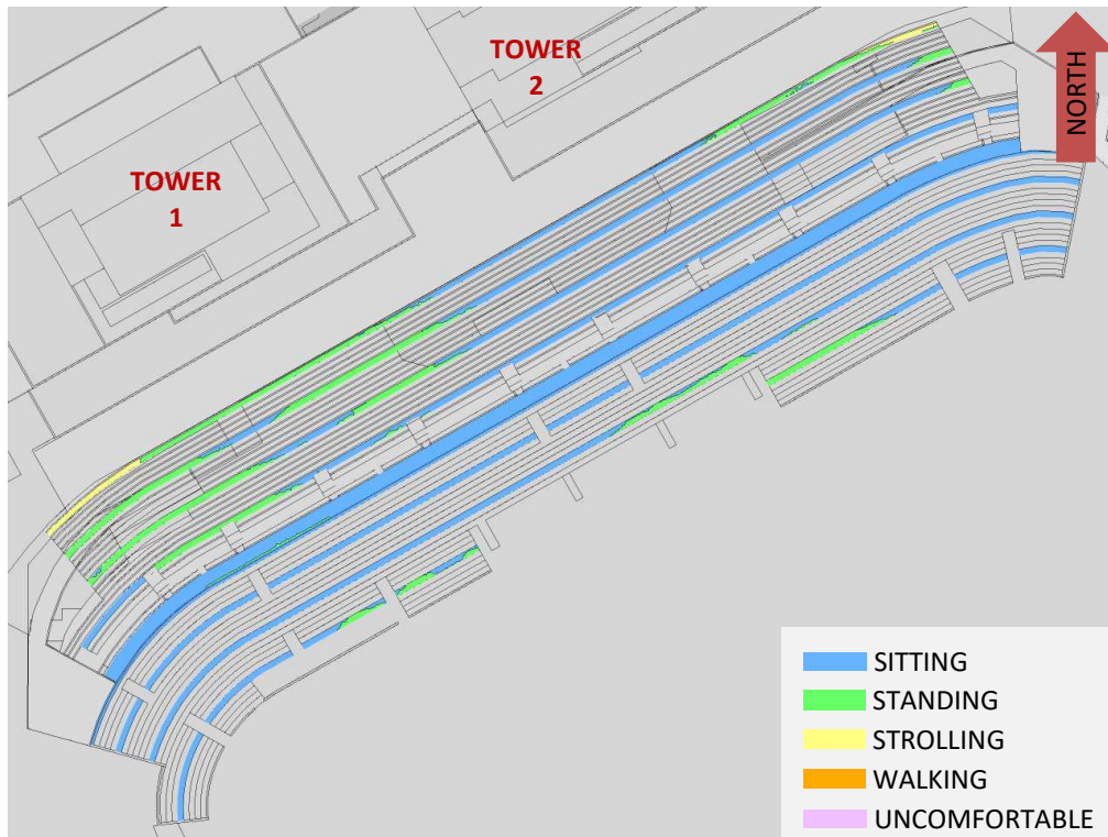
FIGURE 29B: AUTUMN – WIND COMFORT, SELECT NEW NSS ROWS WITHOUT NSS ROOF
