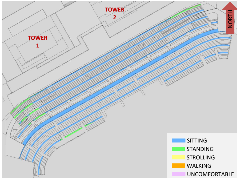
FIGURE 29A: AUTUMN – WIND COMFORT, SELECT NEW NSS ROWS WITH NSS ROOF
