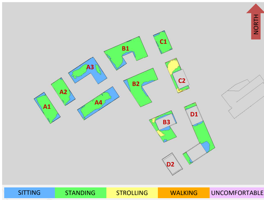
FIGURE 8B: SUMMER – WIND COMFORT, ROOF LEVEL
