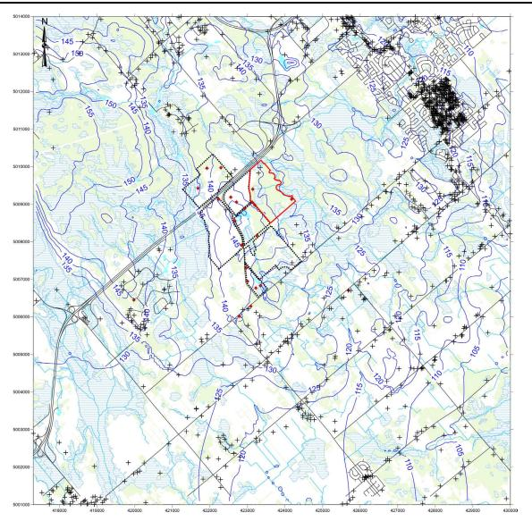
NUMERICAL MODEL SIMULATED WATER TABLE ELEVATION
