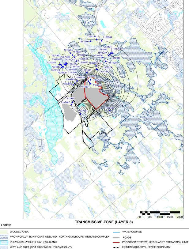
WETLAND AREA (NOT PROVINCIALLY SIGNIFICANT) EXISTING QUARRY LICENSE BOUNDARY SIMULATED GROUNDWATER DRAWDOWN CONTOUR (m) WATER WELL (MECP WWIS) ZONE OF EXTRACTED BEDROCK WITHIN SPECIFIC MODEL LAYER
