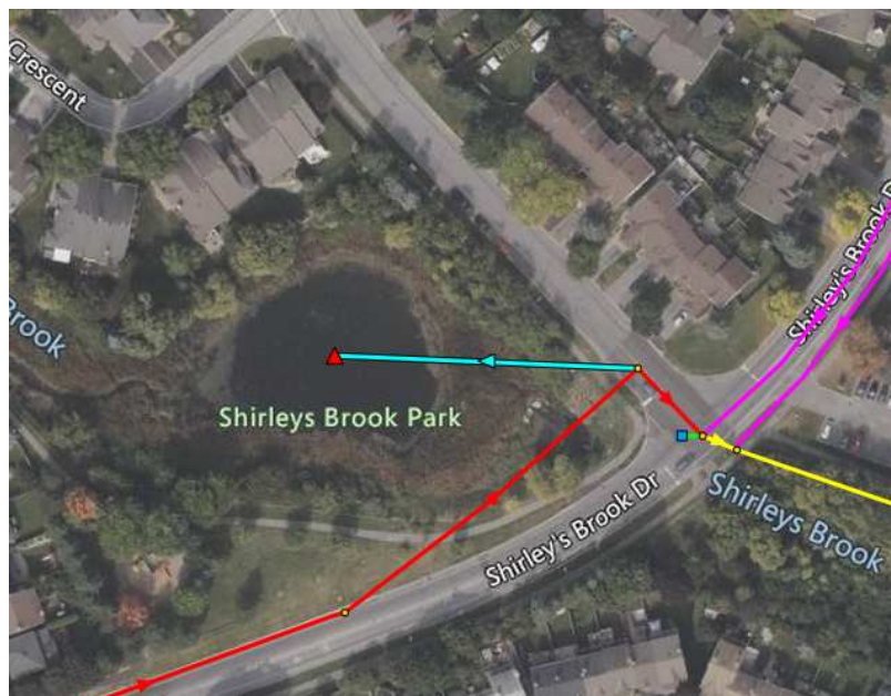
Figure 13: Emergency overflow as modelled in PCSWMM
