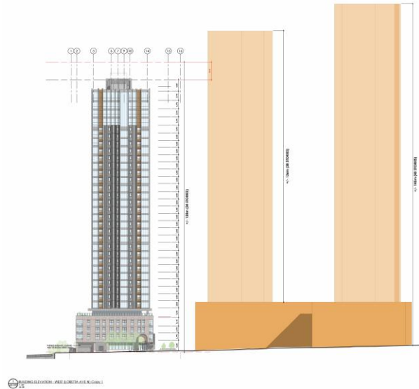
Figure 2: Building Elevations West Massing with the 4-storey podium and the 34-storey tower of Phase 1 setback on the north edge of the site along Loretta Avenue. Phase 2 towers are blocked out, with the podium levels appearing darker than the two towers. Linebox Studio 2025.
