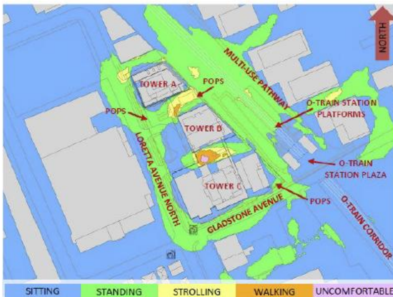
Figure 5: Excerpts from GradientWind's analysis. The Pedestrian Level Wind Study (PLW study) determined the influence of the wind environment on pedestrian comfort over the proposed development site. Their report recommends canopies and specific buffering.
