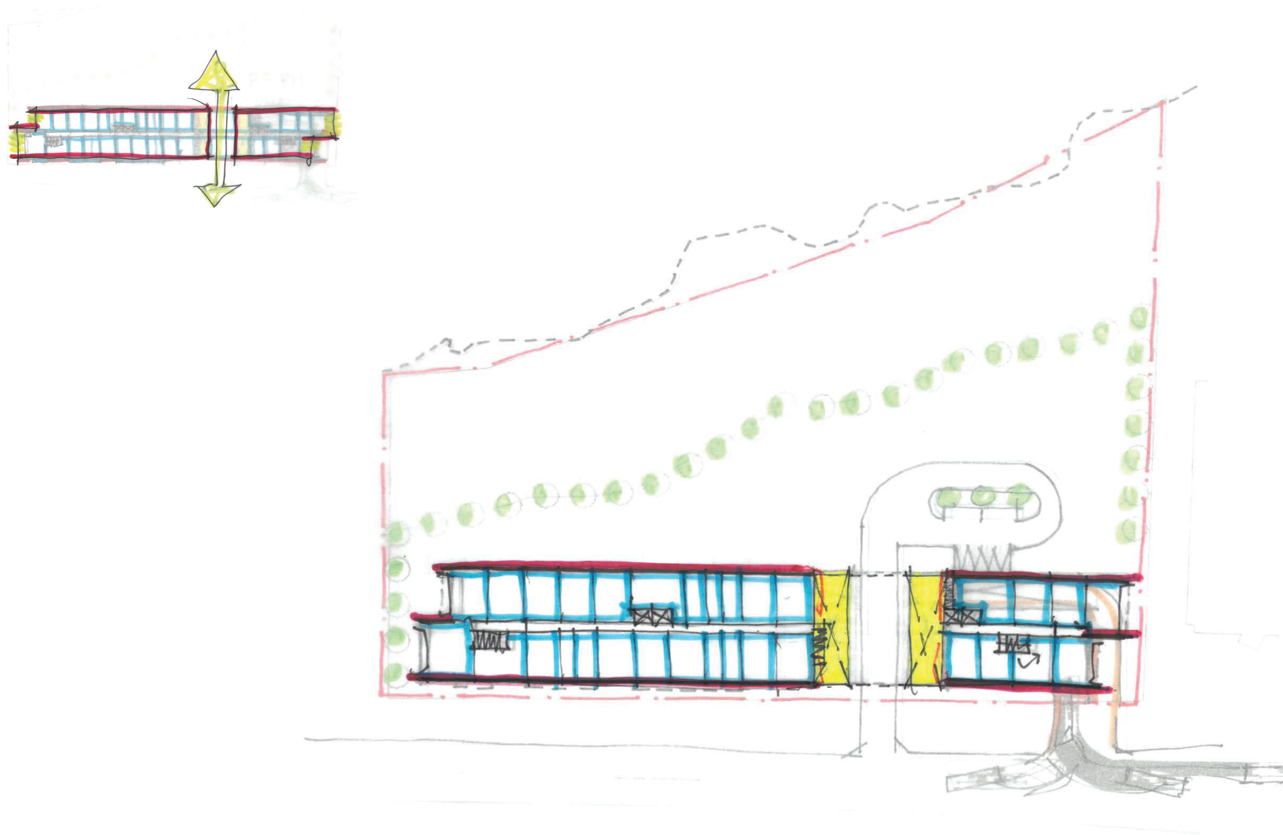
upper left: site parti sketch lower right: plan diagram Level2; yellow area denotes double height main lobby space at either side of breezeway
