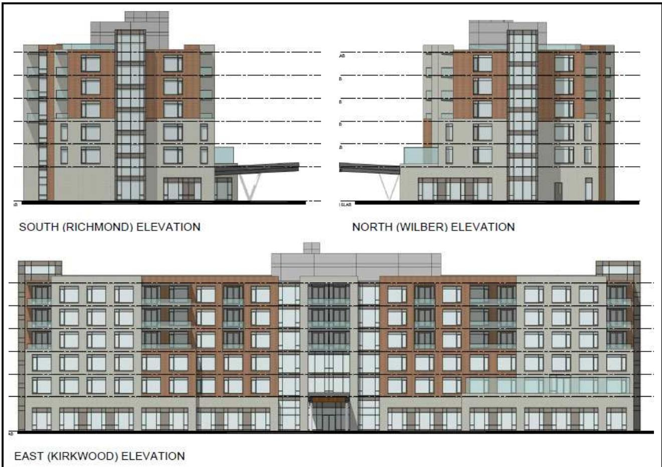
Figure 12. Elevations of six-storey residential building (350 Kirkwood)
