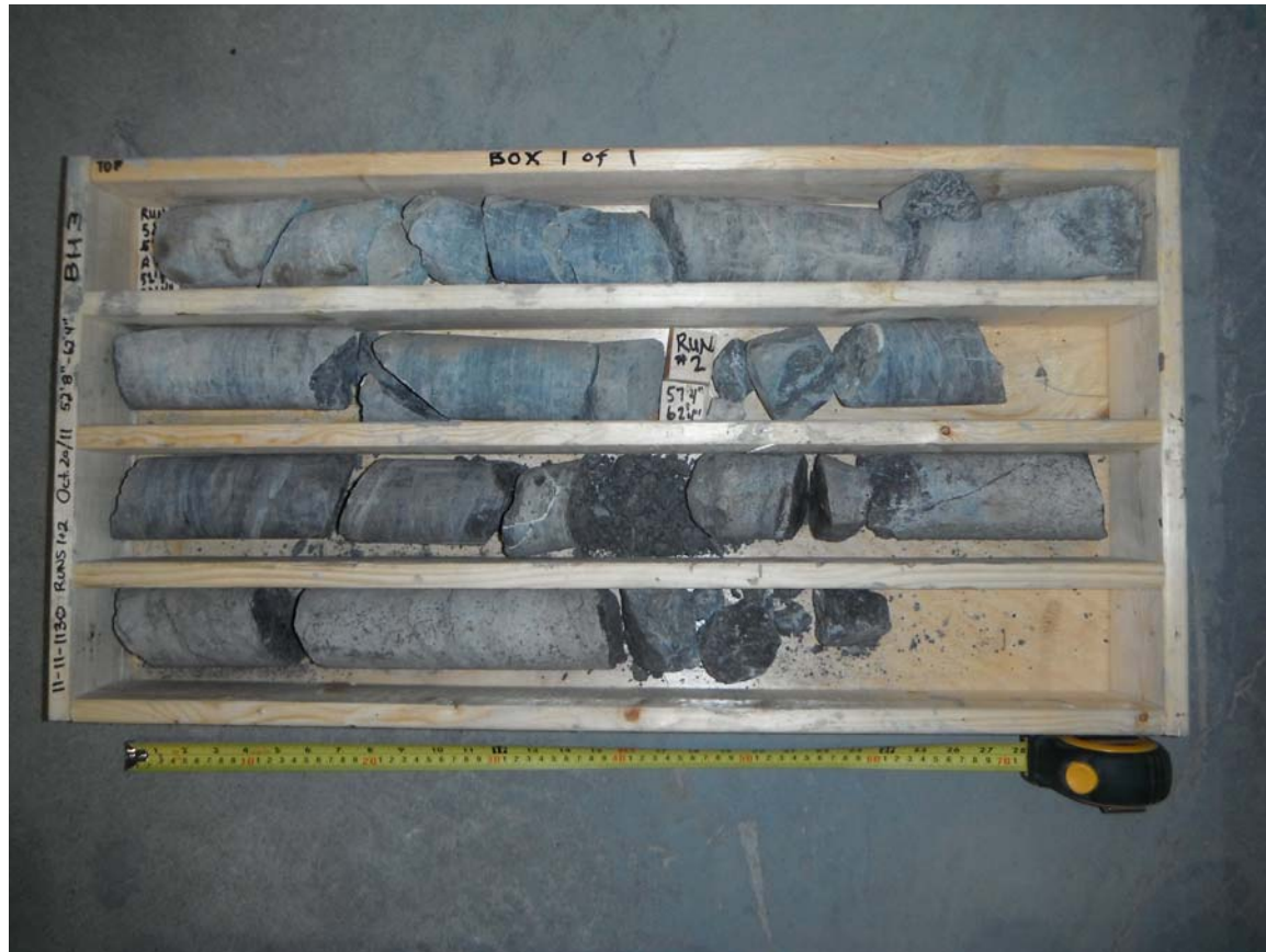
Bedrock Core Sample Borehole: 3 Runs: 1 & 2 Depth: 16.1 - 19.0m (Elev. 83.1 – 80.1 m)
