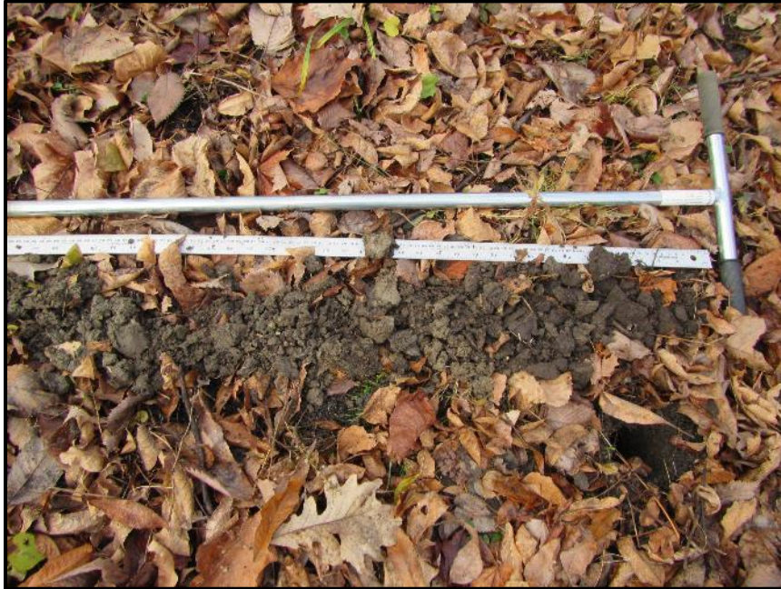
Photograph 3: Soil profile in Fresh to Moist Green Ash Lowland Deciduous Forest. Silty Clay Loam material shown (November 16 th , 2016).
