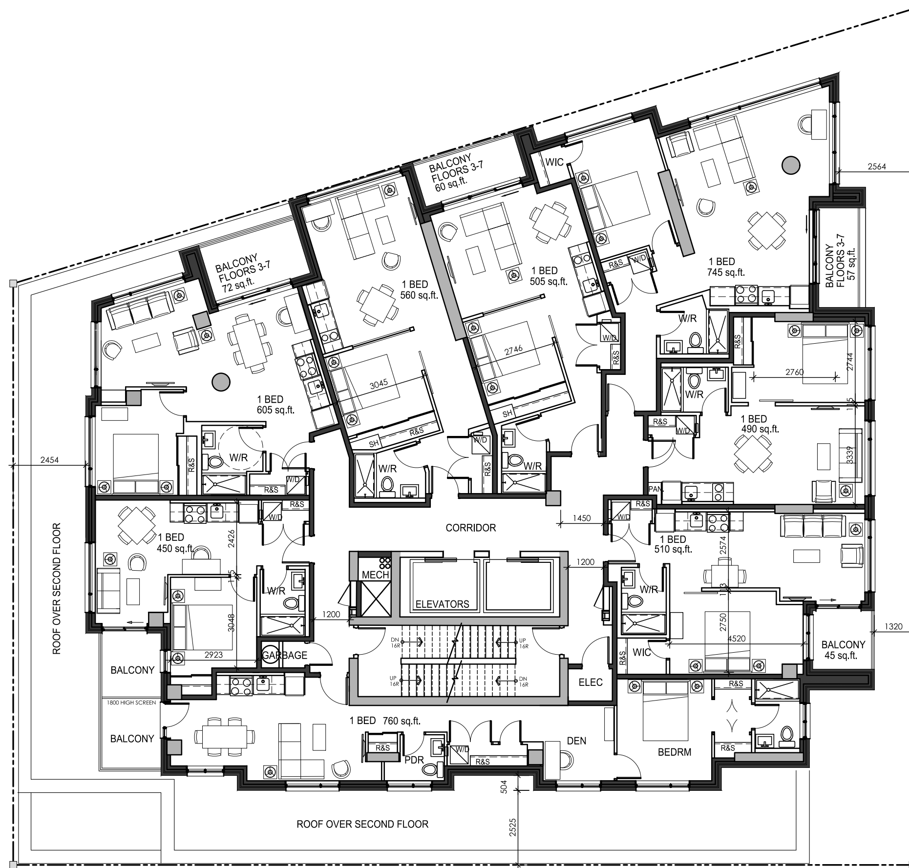
5 4TH - 8TH FLOOR FOR PROPOSED 14 STOREY TOWER - 8 D.U. PER FLOOR - GROSS AREA = 5485 SQ.FT. SCALE: 1:125
