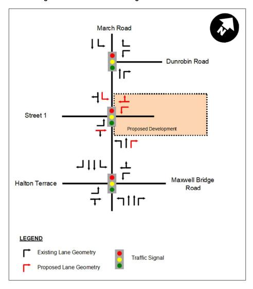
Figure 15 - 2031 Total Lane Configuration and Traffic Control
