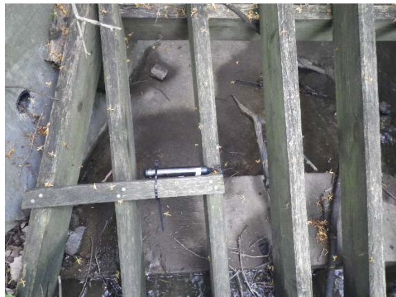
Figure 2d: Barometric Logger Installation at Q3
