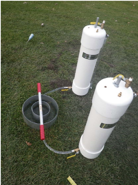
Figure 2: Double-Ring Infiltrometer Setup (15/30 cm rings, two Marriotte bottles)
