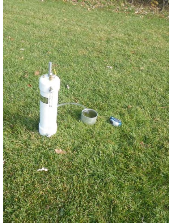
Figure 3: Single Ring Infiltrometer Setup (12.7 cm diameter steel ring, single Marriotte bottle)
