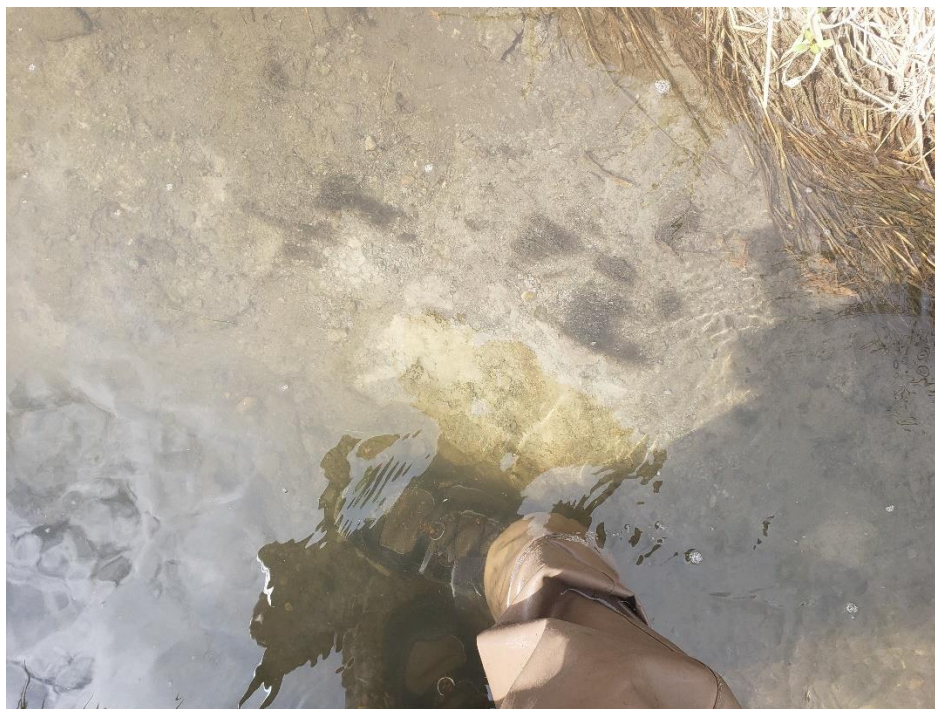
Exposed compact grey clay was frequently observed along the bed of the channel.
