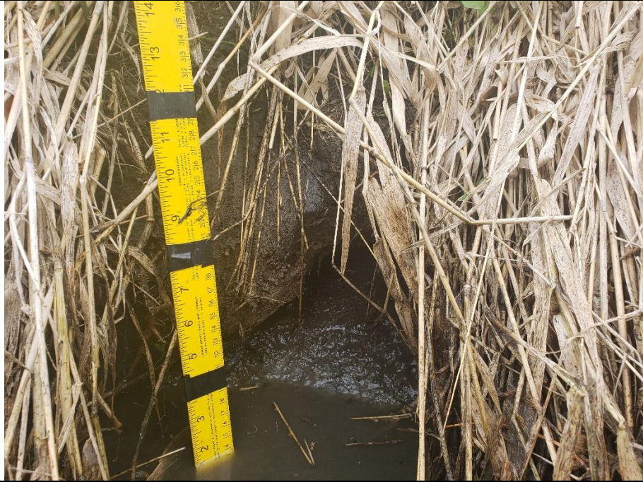
Below the dense grass rooting structure, both banks through the natural riparian area of KDR-4 are composed of a loamy clay.
