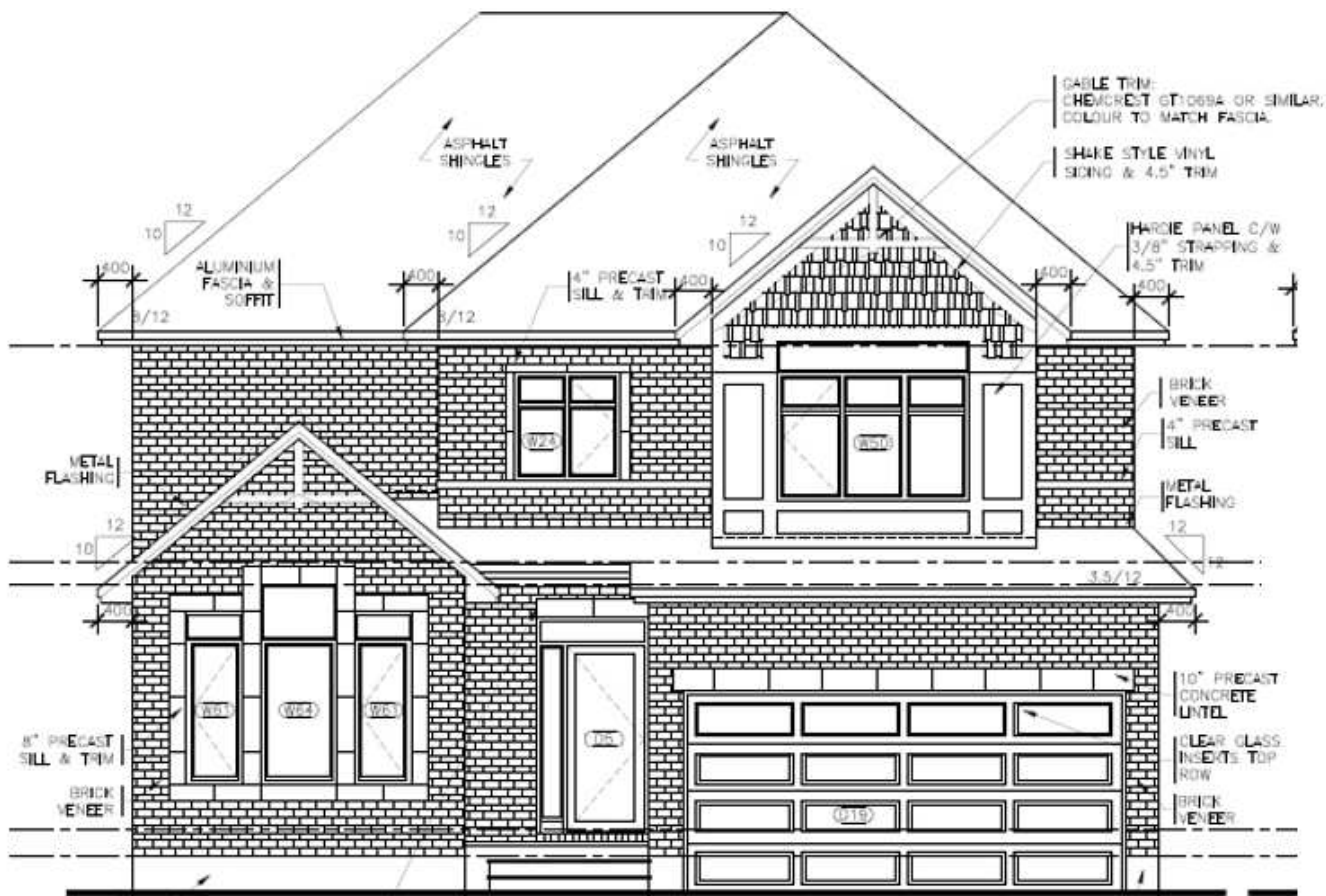
Figure 6: Typical front elevation drawing of a proposed dwelling unit model
