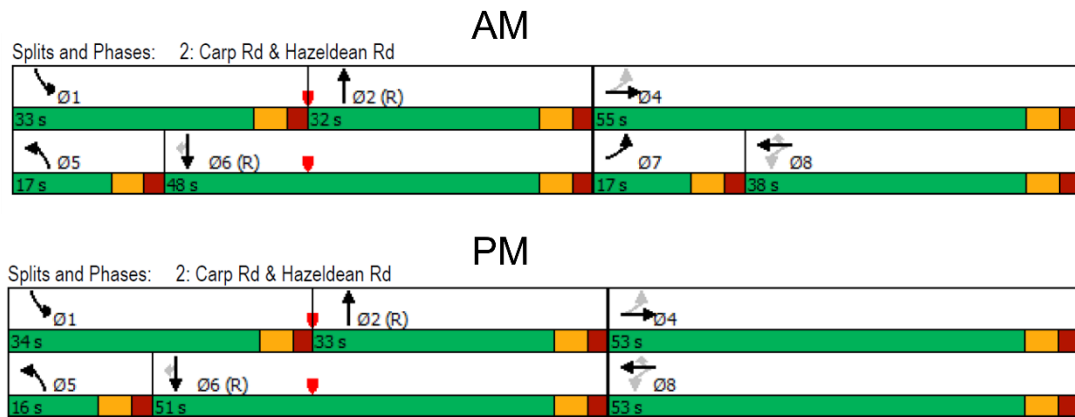
Figure 15 – Carp Road & Hazeldean Road Optimized Signal Timings
