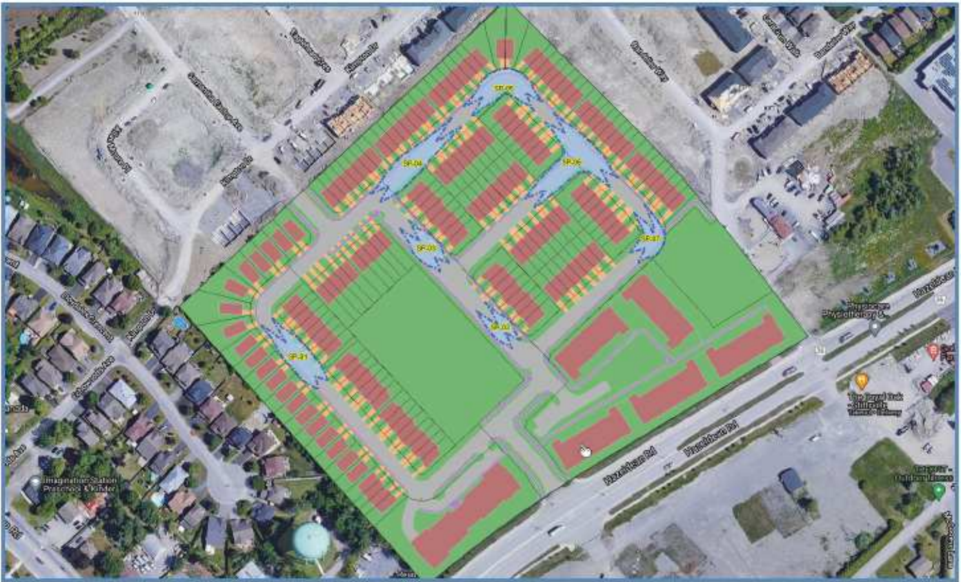
Figure 7-1: Surface Ponding Locations
