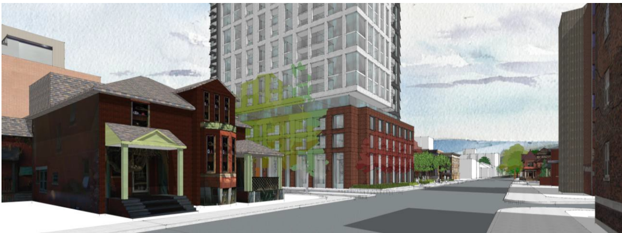
Figure 24: Traditional red brick for the podium, its height and the setback treatment between it and the body of the tower help ground the development. Source Hobin Architecture August 2020.
