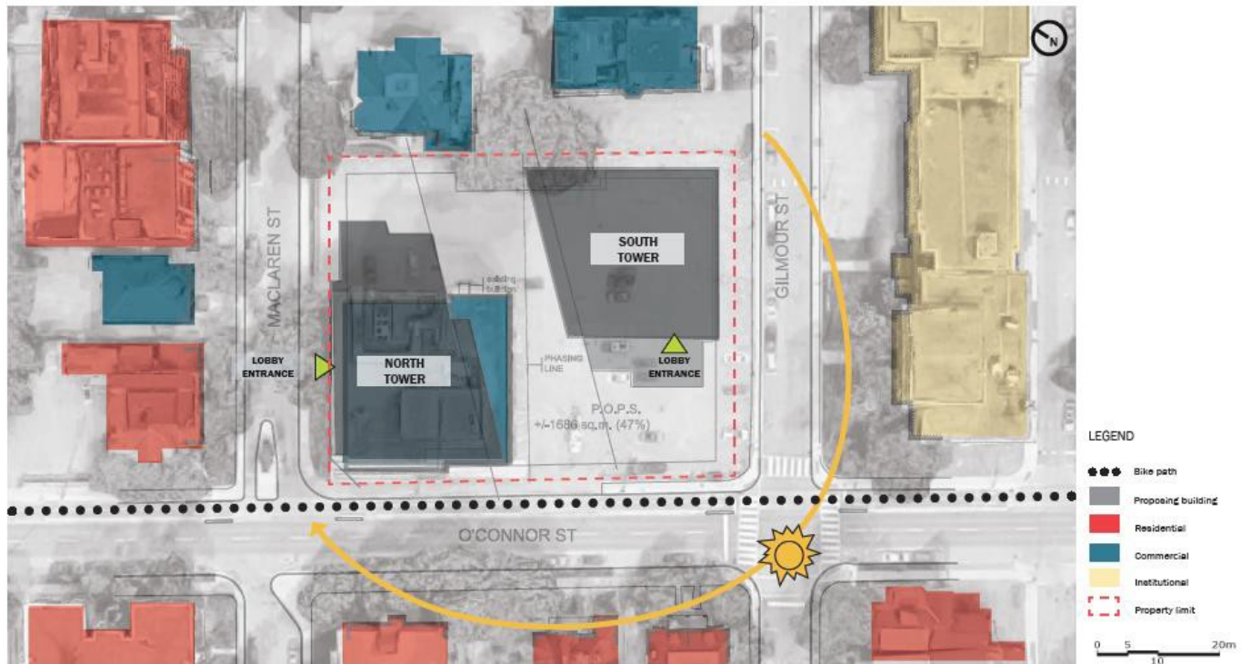
Figure 18: The placement of the two towers on the lot takes advantage of the southern exposure. Both towers are positioned proud of the setback of existing heritage buildings along MacLaren and Gilmour Streets. Source: Projet Paysage 2020 .
