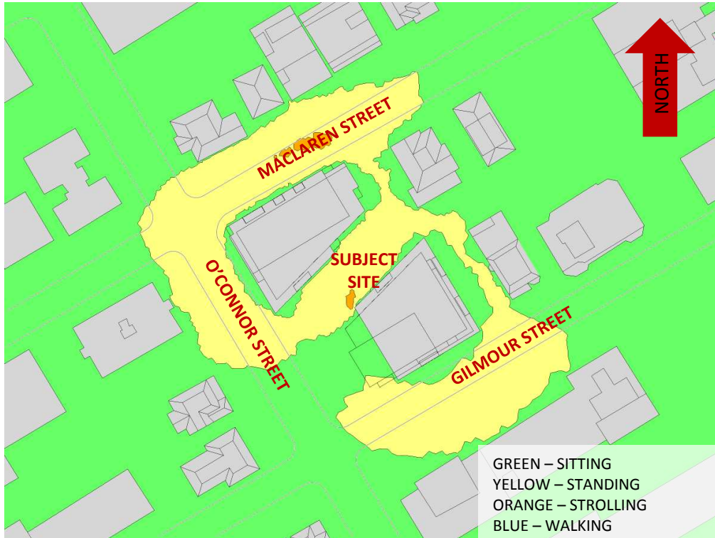
FIGURE 3C: AUTUMN – WIND CONDITIONS AT GRADE LEVEL
