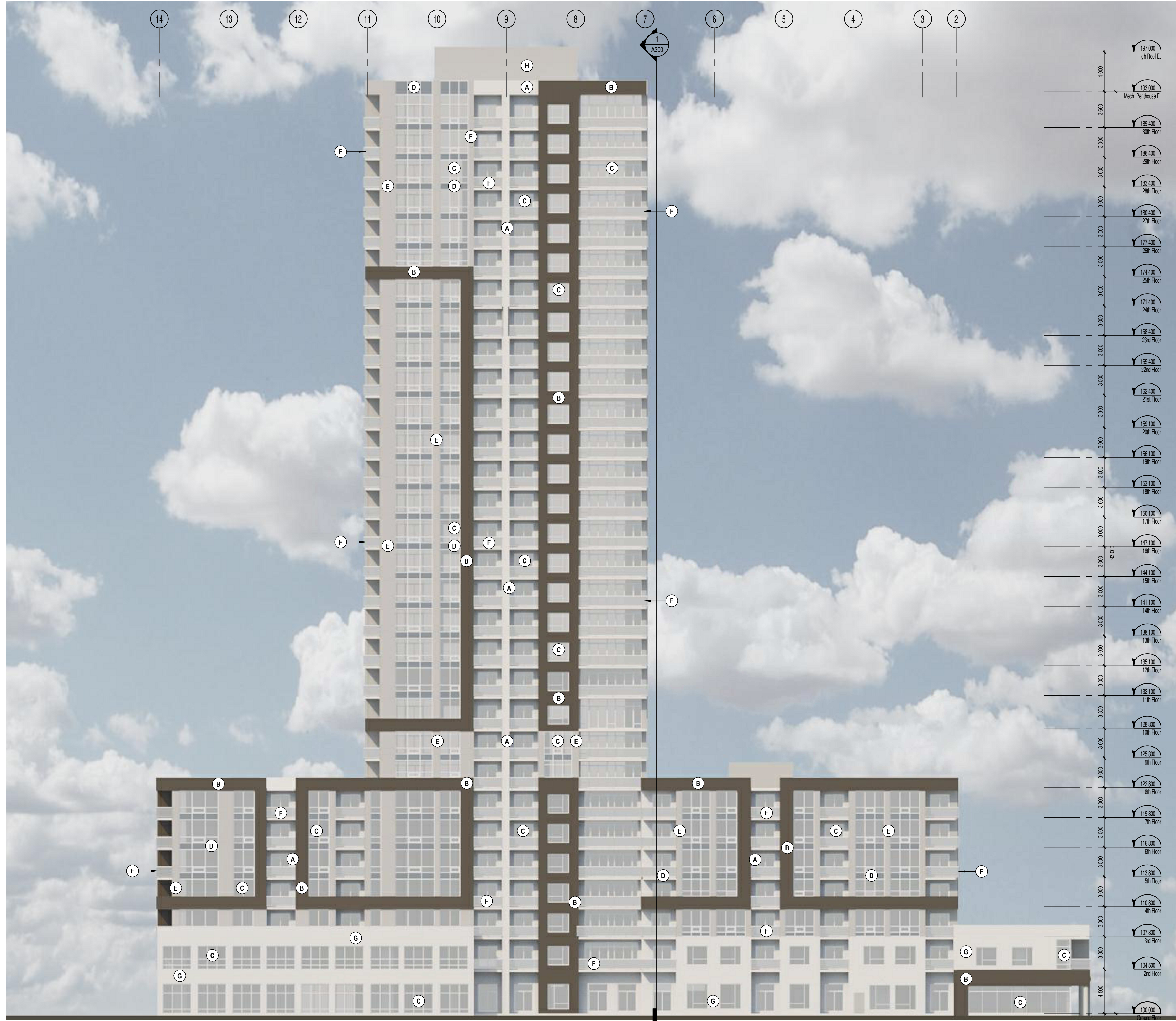
EAST TOWER - East Elevation 1 : 200
