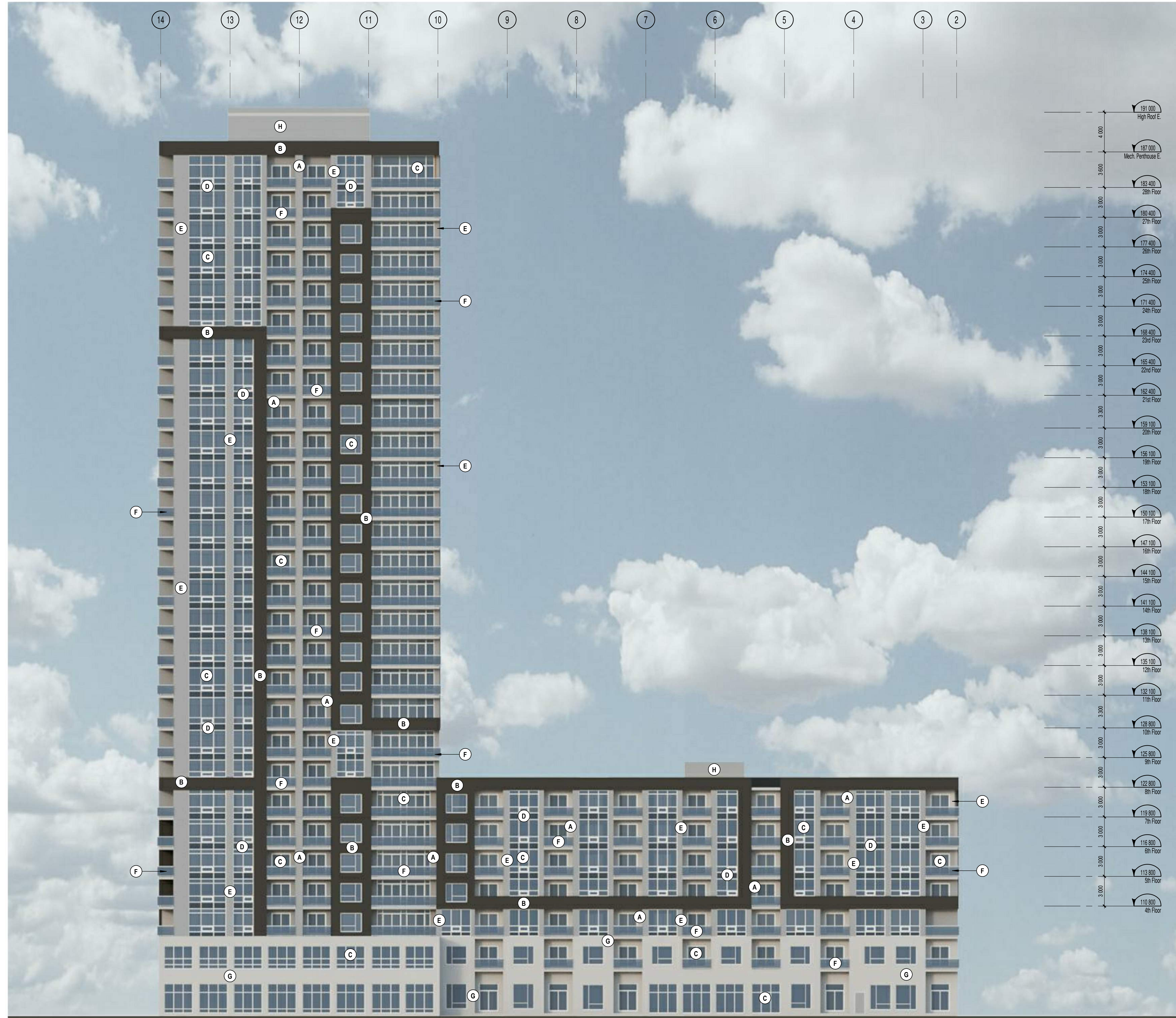
EAST TOWER - East Elevation 1 : 200
