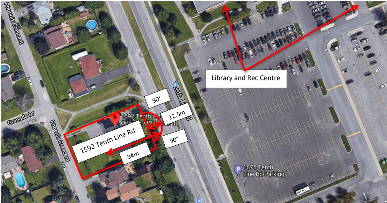
Figure 2.2 – Surrounding area 1592 Tenth Line Road with locations, distances and angles of relevant noise sources
