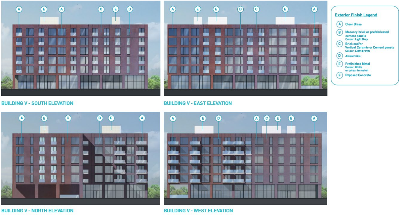
Figure 34. Building V design details.
