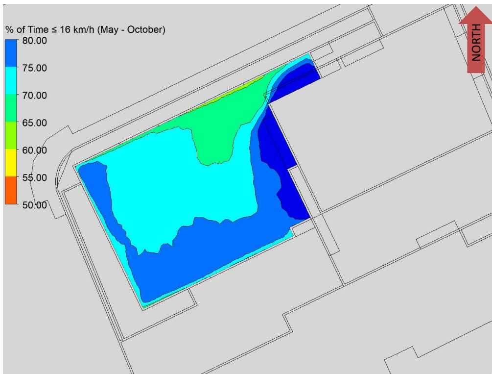
FIGURE 8B: PERCENTAGE OF TIME SUITABLE FOR SITTING IN FIGURE 8A
