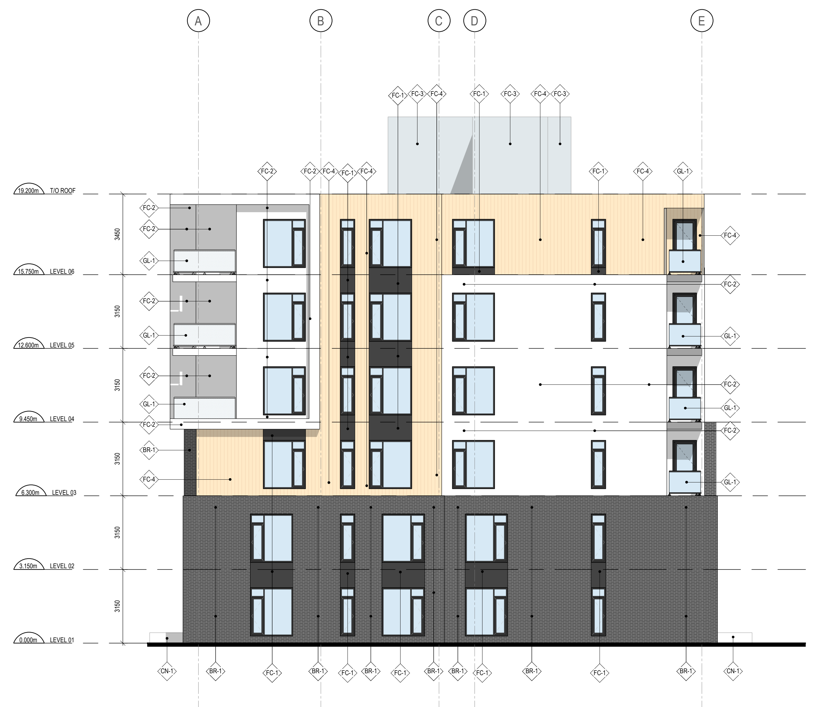
1 WEST BUILDING - WEST ELEVATION A206 SCALE: 1 : 100
