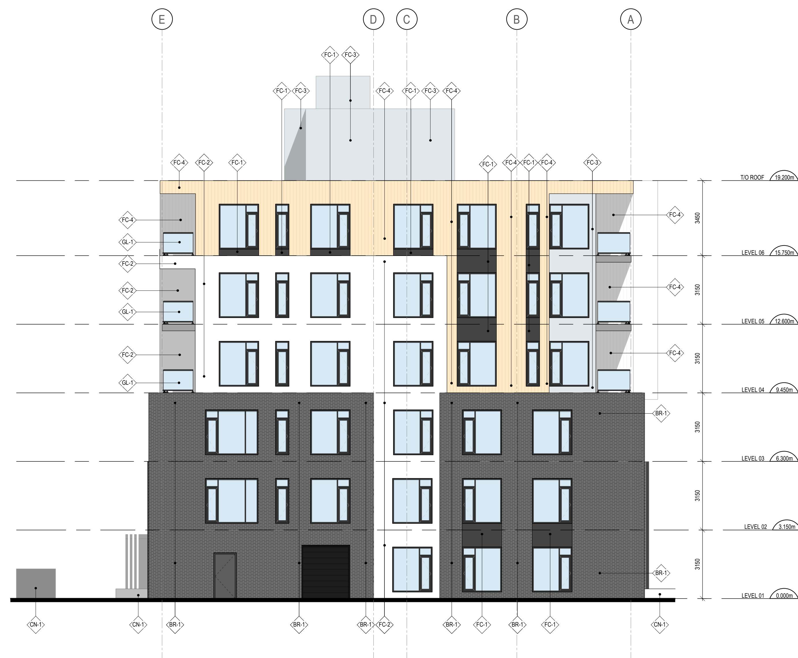
2 WEST BUILDING - EAST ELEVATION A206 SCALE: 1 : 100
