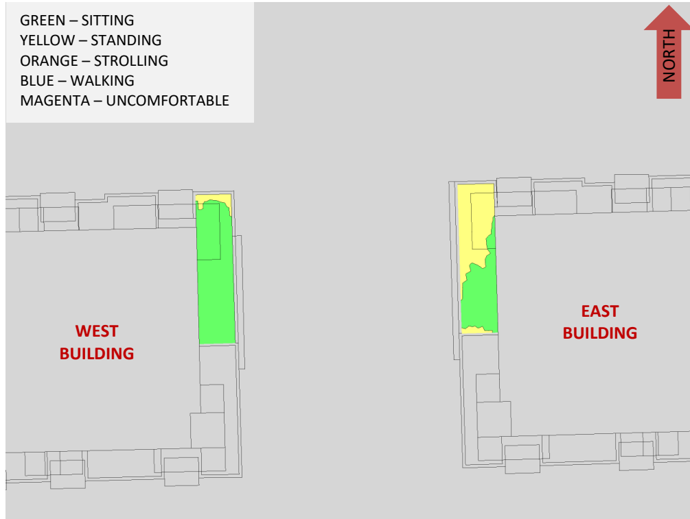
FIGURE 5A: TYPICAL USE PERIOD – WIND COMFORT, AMENITY TERRACES (LEVEL 5)
