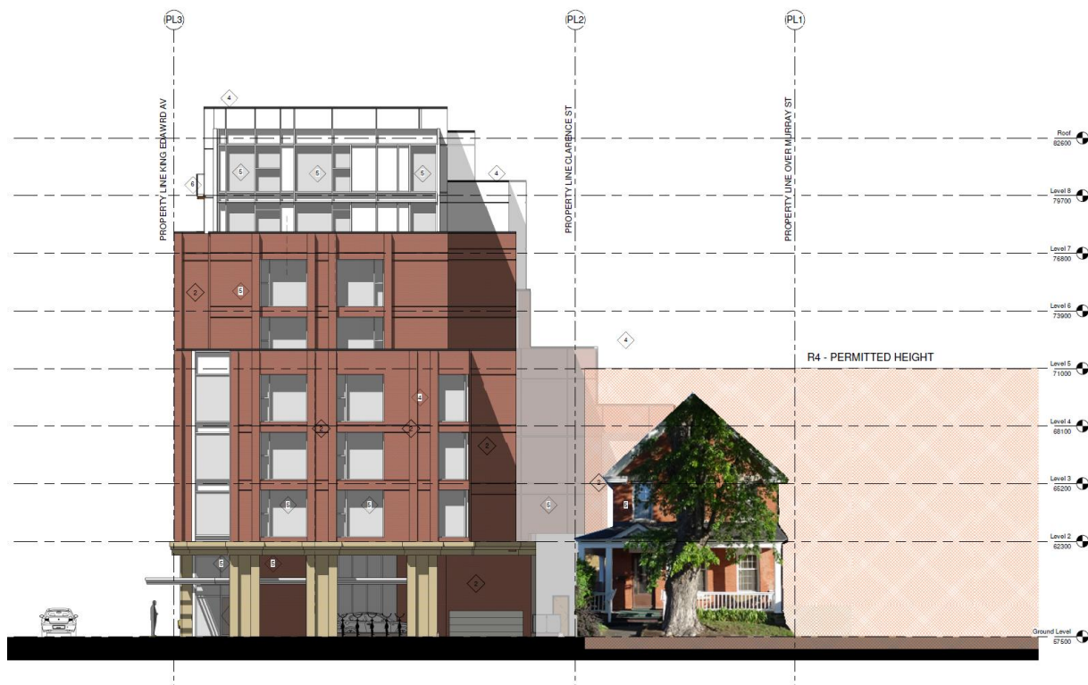
Figure 12: The main entrance to the hotel is located at the corner of King Edward Avenue and Clarence Street where the first floor is set back from the property line with the enclosed entrance to the underground garage set back approximately 11 metres to accommodate the wrap around verandah on the adjacent property and is setback from the neighbouring property.
