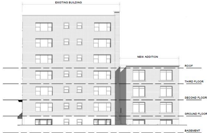
Figure 9: South Elevation of the proposed addition
