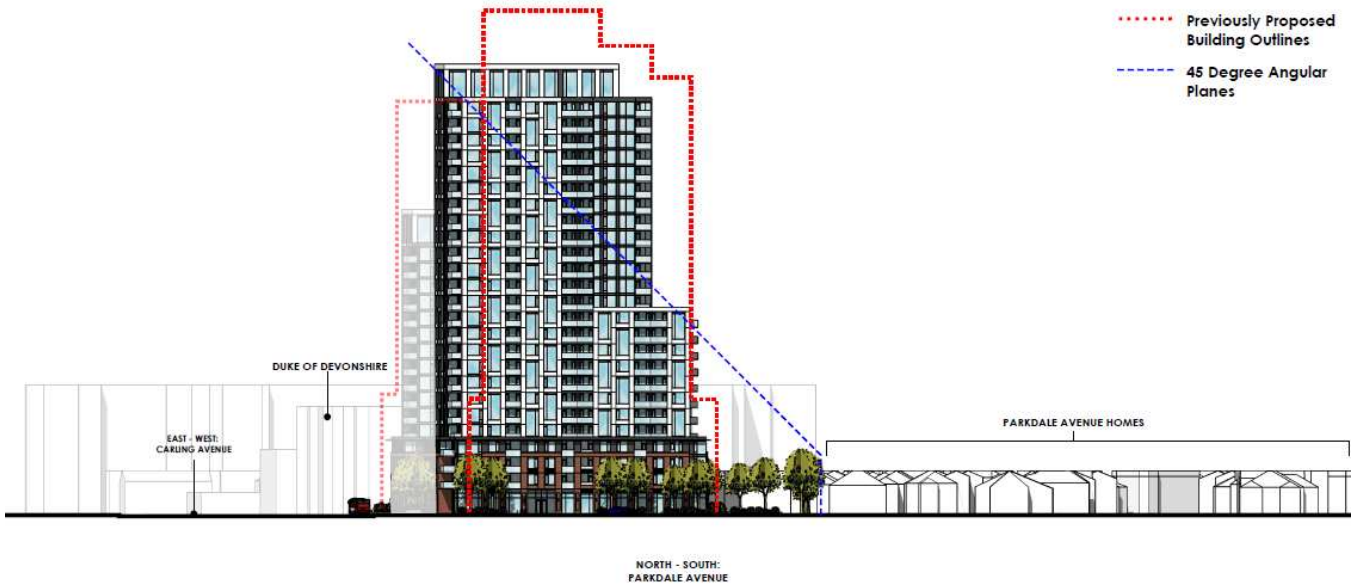
Figure 2: Transition from the subject site to the low-rise community to the north, looking west on Parkdale Avenue
