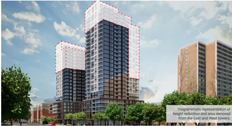
Figure 29: diagrammatic representation of height reduction and area removed from the East and West towers as well as the reduced massing illustrates efforts to minimize shadowing. The white areas of both towers illustrates the portion of each building that has been eliminated.
