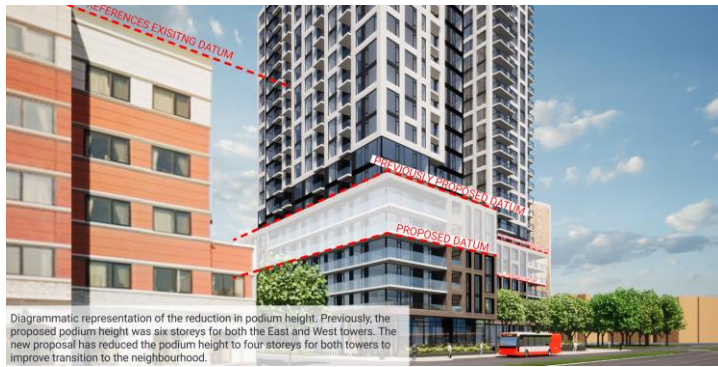
Figure 27: Diagram illustrating the reduced podium height from 6 to 4 storeys.
