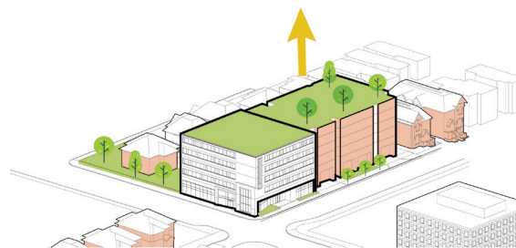
(3) Podium height references existing Legion building height and creates transition to the abutting neighbourhood - Elevate green space - Open ground floor of Legion to recreate a two-storey ground plane and increase site porosity
