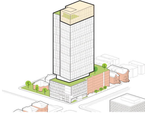
(6) Three-storey grid provides high performing building envelope due to limited glazing - Architectural language extends to the crown to encapsulate mechanical equipment, shade rooftop terrace, and create skyline impact
