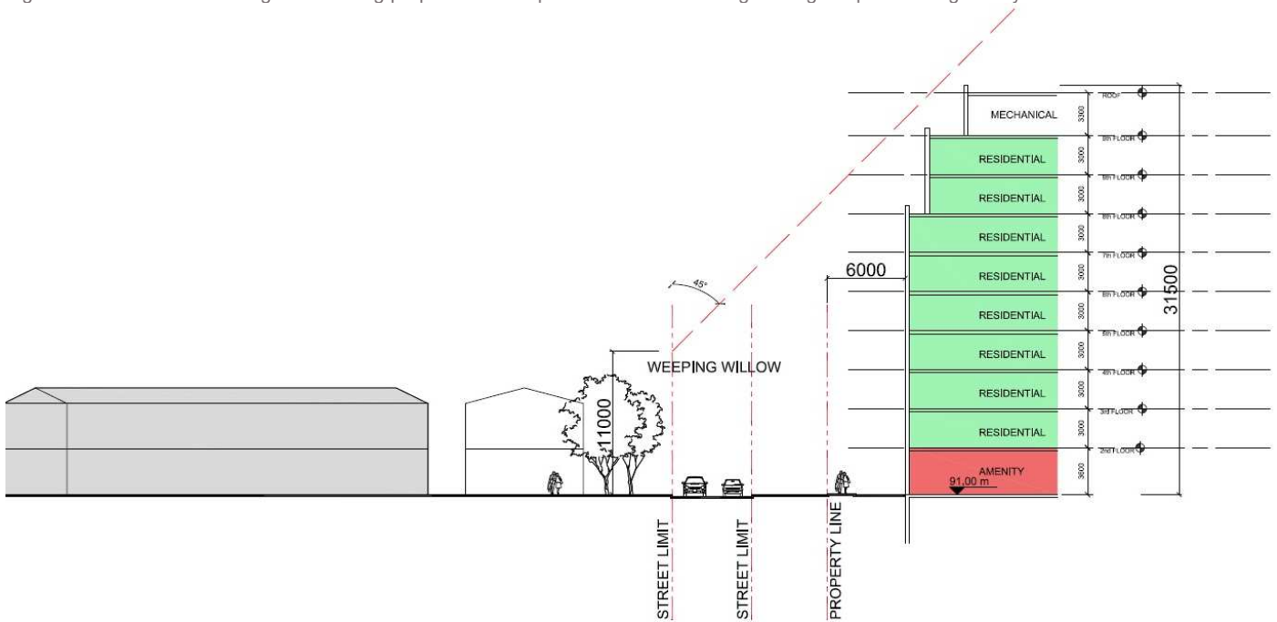
Figure 11: Cross Section Diagram showing proposed development within the 45 degree angular plane along Weeping Willow Lane
