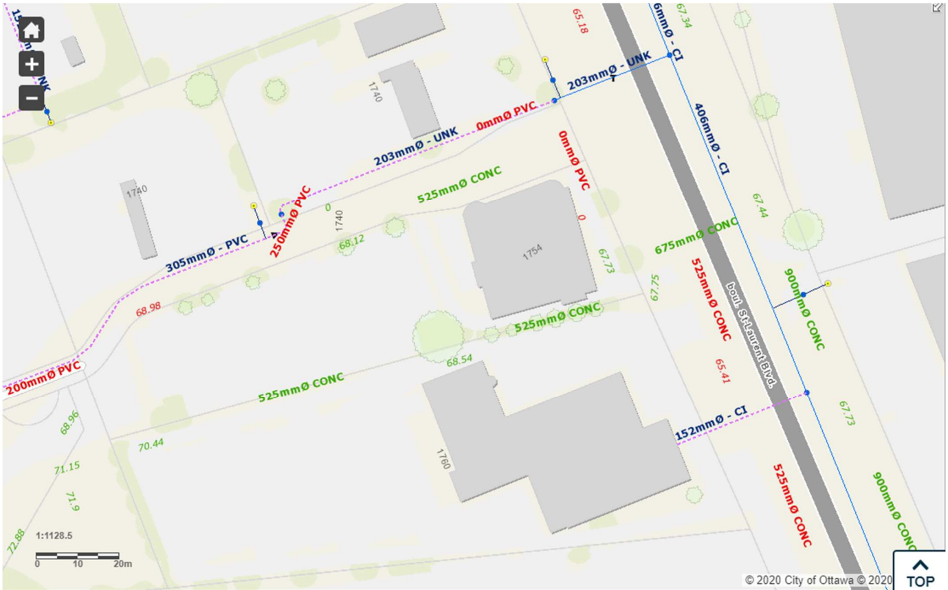
Figure 5-1 – Water Servicing for Existing Buildings
