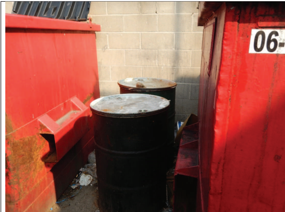
Photo 26: View of the drums use to store the grease collected from the grease trap, no staining observed (facing north)
