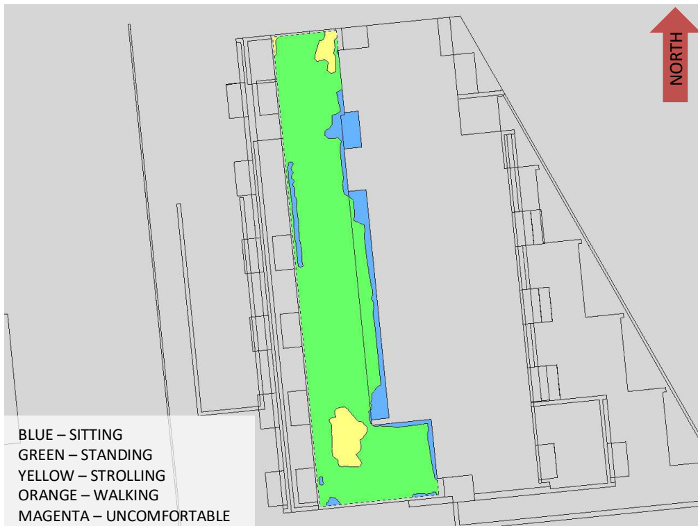
FIGURE 4D: WINTER – WIND COMFORT, LEVEL 17 AMENITY TERRACE
