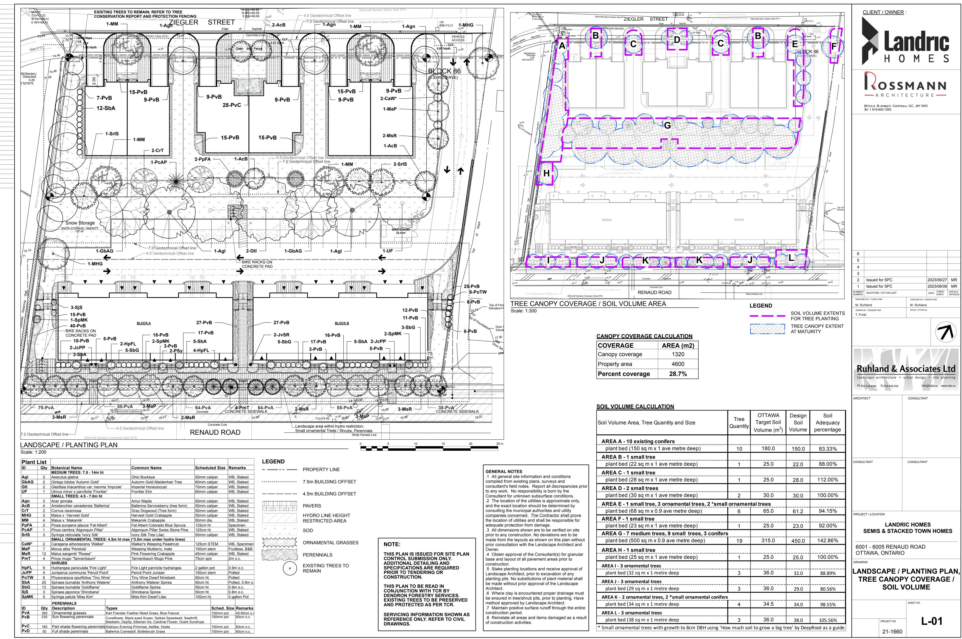
TREE SOIL VOLUME REQUIREMENTS: STANDARD TREE SOIL VOLUMES QUANTITIES INCLUDE THE TOP 900-1000mm OF SOIL/EXISTING SUBSOIL LAYER TO CALCULATE TOTAL SOIL VOLUMES REQUIRED BY CITY OF OTTAWA FOR SUSTAINABLE TREE GROWTH. WHERE LARGER SOFT AREAS ARE AVAILABLE, THE TOP 400-500mm LAYER IS USED TO CALCULATE SOIL VOLUMES.
